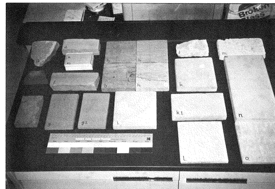
Similarly this group of sandstones and limestones from the United States again illustrates rich diversity. (b) and (c) are Bluestones from the Catskills, New York State. Two samples marked (e, e1) are Scioto sandstones from Ohio. Four examples marked (h) are Briar Hill sandstones from Ohio. (i) is a Berea sandstone from South Amherst, Ohio. (k, k1) and (n) are Indiana limestones with various finishes. (m) is a Texas shellstone, a fossiliferous limestone.
