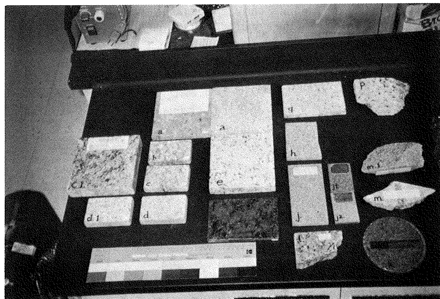
This group of granites from the United States shows the great diversity which is to be found even within such a small selection. (a) and (e) are Stoney Creek granites from Rhode Island. (c, c1) Grey Tapestry granite from the Baretto Granite Corp. New Hampshire. (f) is a Cold Spring Granite Co., Spring Green (i, j1, j2) are Westerly blue, light and pink granites from Rhode Island. (l) is a Cold Spring Texas Red granite. (m) is a Barre blue grey granite from Vermont.
