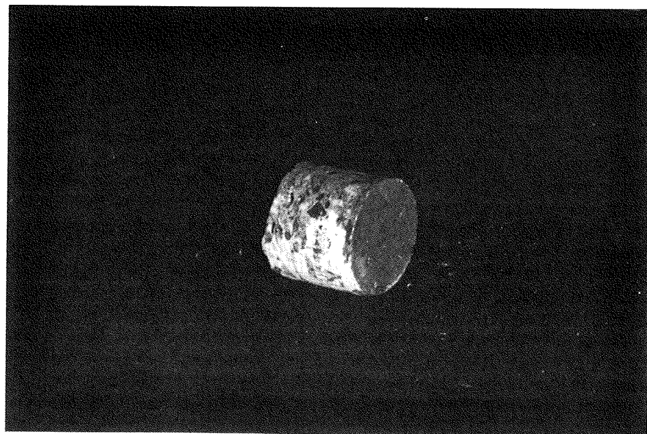
This core from some historic concrete has been coated with an epoxy resin which has consolidated the concrete but has radically changed its appearance making it darker, yellow and glossy.
